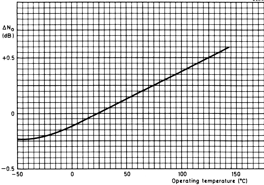
Typical change in noise figure as a function of temperature
